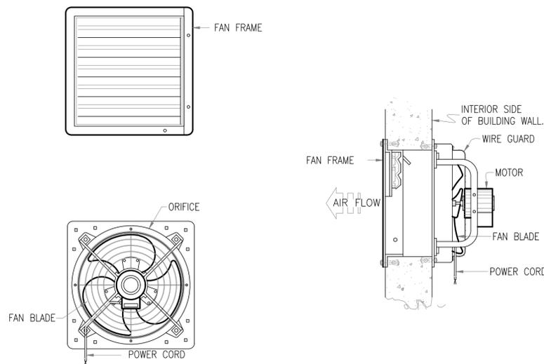
**PROPELLER EXHAUST FAN INSTALLATION DETAIL**
